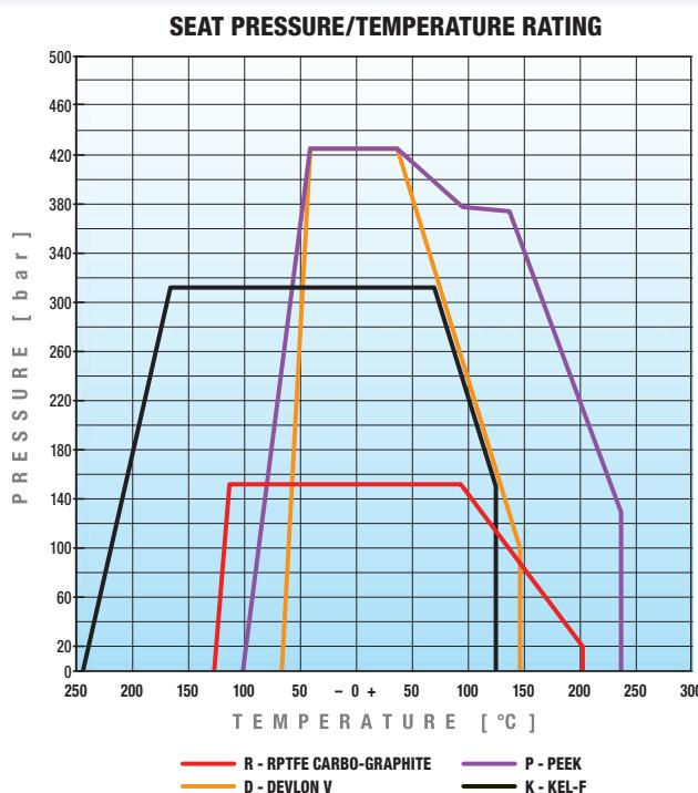
Choosing the right seat material is the most important decision in ball valve selection. Use the Pressure/Temperature rating chart for the most common seat materials and ask us in case of special material or applications.
